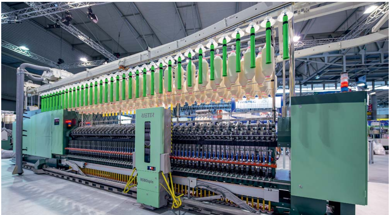
Already successfully in use: the piecing robot ROBOspin, which repairs ends down and thus ensures high productivity.
