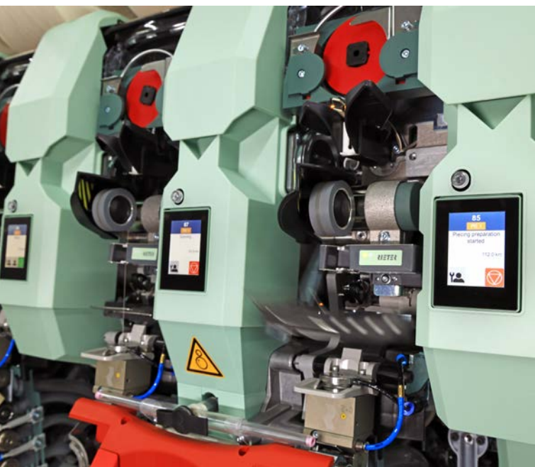
Fig. 4: Simplified operation – one display per spinning unit
