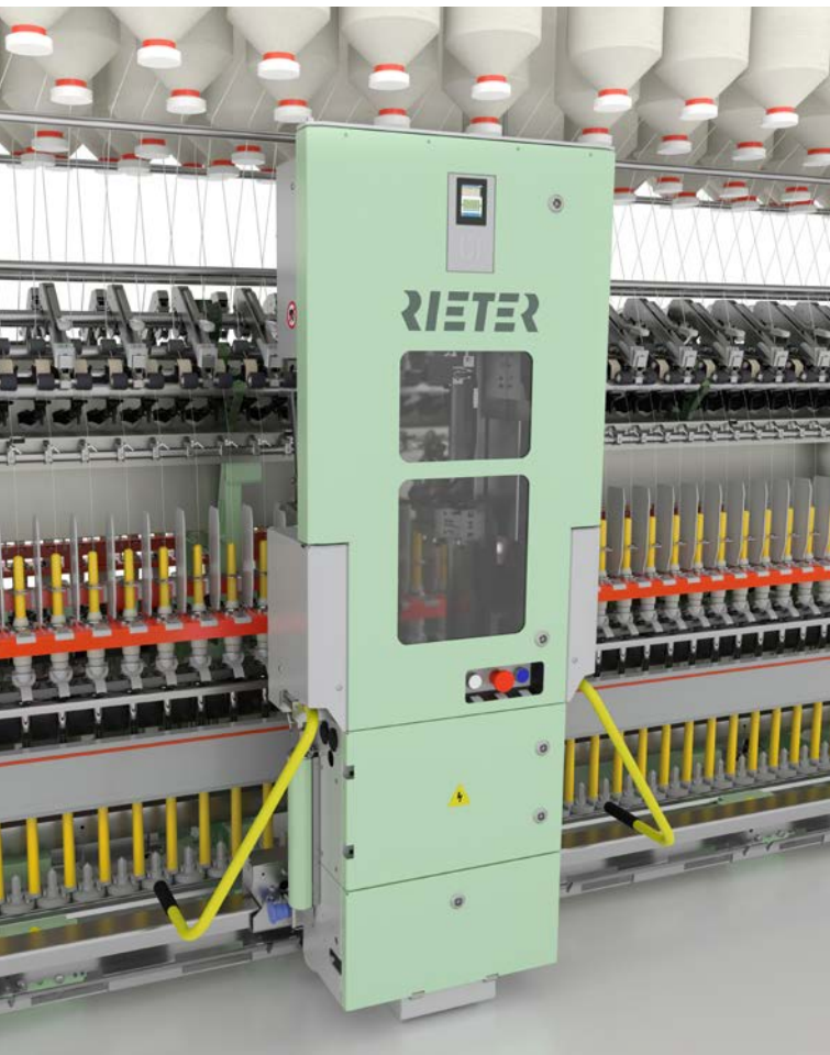
Fig. 1: ROBOspin on a Rieter ring spinning machine G 38
