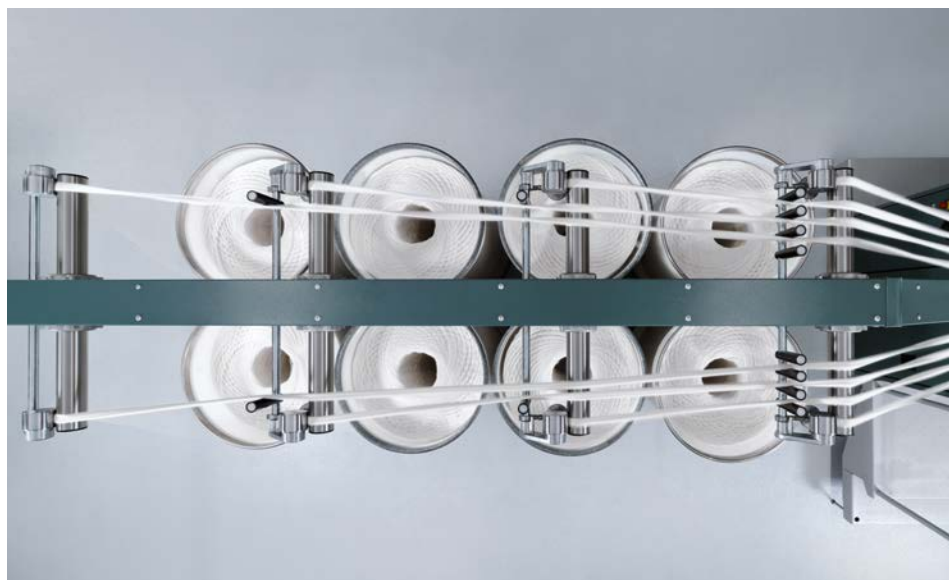
Fig. 2: Reinforced power creel for enhanced robustness
