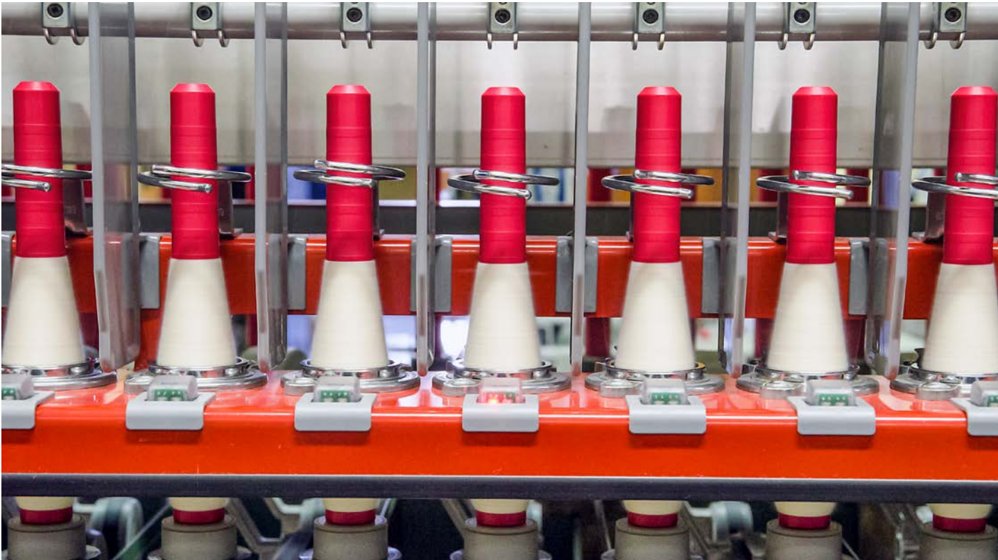
Fig. 3: The individual spindle monitoring system ISM detects the affected spinning position.
