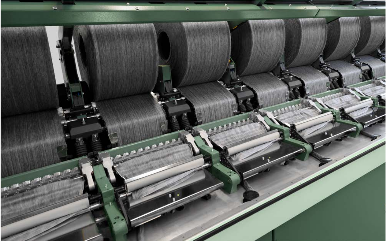
Fig. 1: Disturbing short fibers and neps are combed out with the comber E 90.
