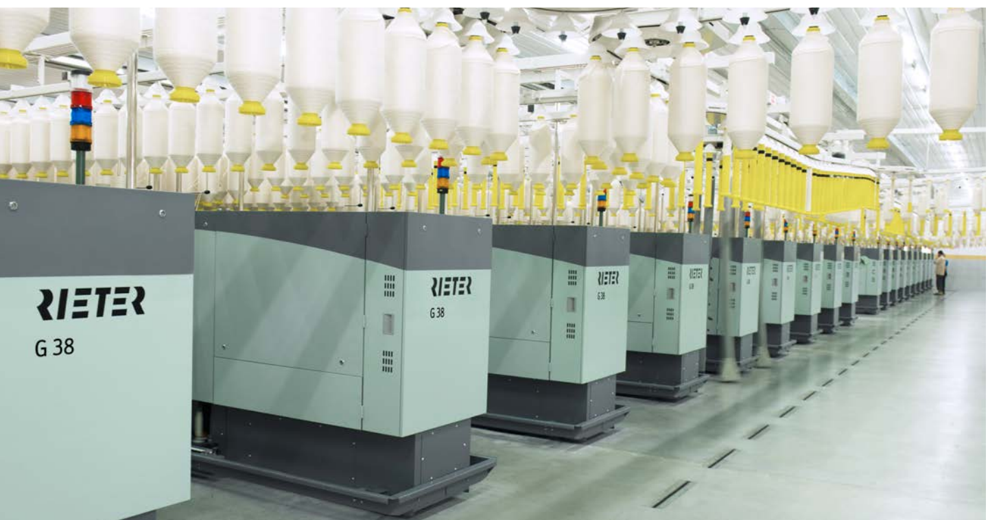
Fig. 1: The proven ring spinning machine G 38 achieves up to 15% higher yarn production with the High-Speed Package.
