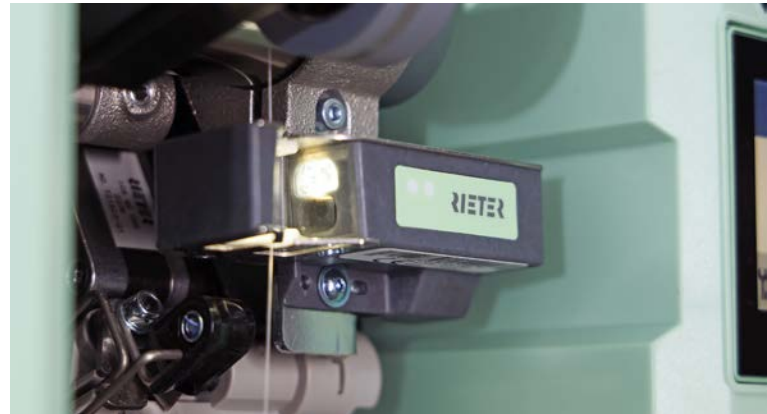
Fig. 5: Yarn clearer Q 30A – effective quality control for air-jet spun yarns
