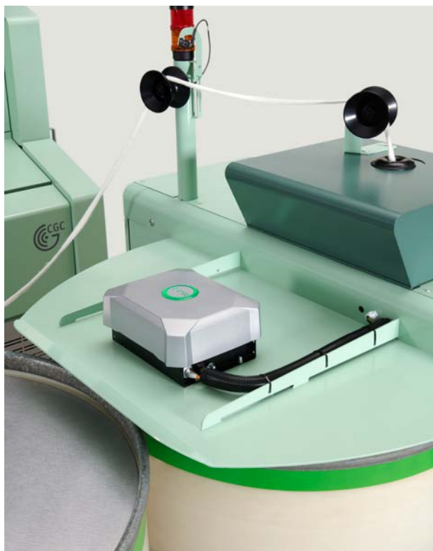
Fig. 2: Trash level monitor at the sliver coiling section of the card
