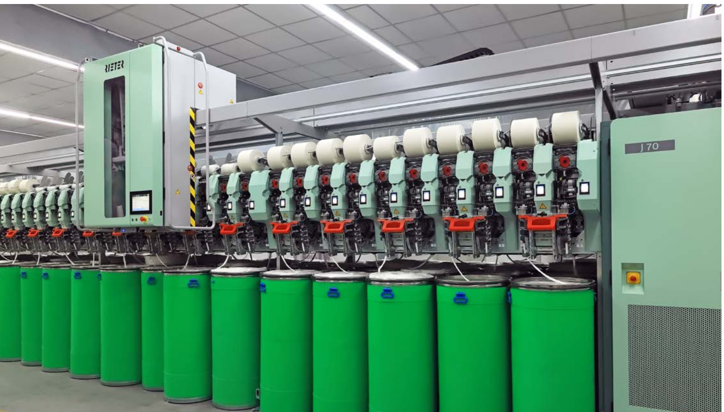
Fig. 1: The air-jet spinning machine J 70 with individually automated spinning positions
